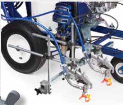
Dual Wing Nut Design for separate vertical and horizontal adjustments
